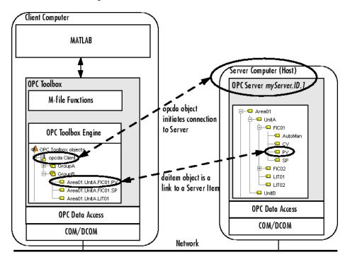
The opcda client object establishes the connection between MATLAB and the OPC server, using OPC Data Access Specification standards. The standards are based on Microsoft COM/DCOM interoperability standards.
