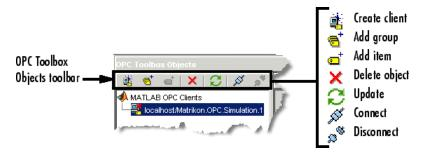
Click **Connect** in the **OPC Toolbox Objects** toolbar. If the client is able to connect to the server, the icon for that client in the **OPC Toolbox Objects** tree will change to show that the client is connected. If the client could not connect to the server, an error dialog will show any error message returned. See "Troubleshooting OPC Issues" on page 1-17 for information on why a client may not be able to connect to a server.
