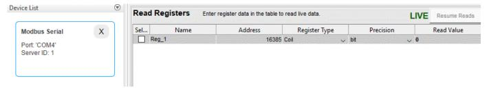
7 You then use the table to set up more reads from your device. Fill in the **Read Registers** table to read data from two timers and three switches. Since the table automatically displays the register you configure in the **Configure** tab, the first timer is already listed. Change the name to C1, then add four more rows so you have these reads set up.
