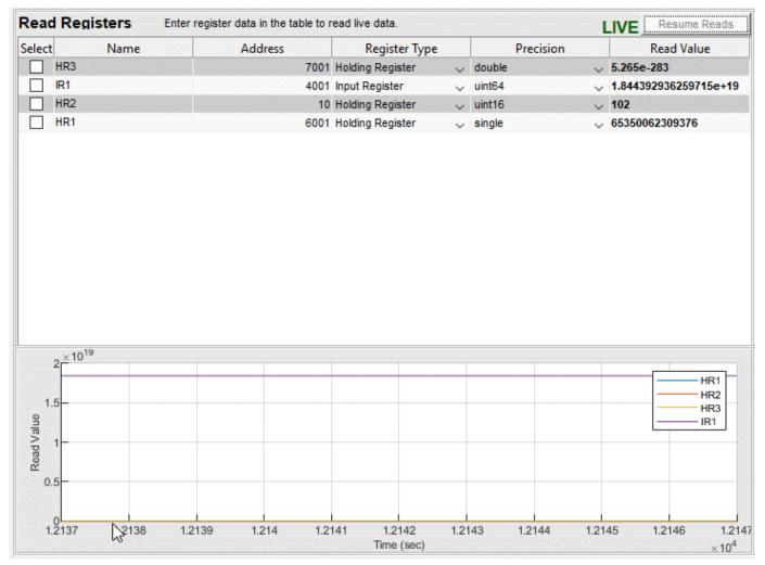
If you want to alter the plot, use the **Plot Tools** section. You can change the axes, show or hide the legend, and select which registers to display in the plot. The plot changes dynamically when you change any of these factors using the plot tools.
