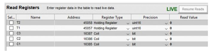
In this case, the value of 0 means the switch or timer is connected and available, but it is not activated.
